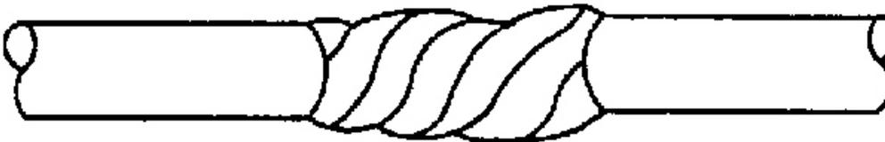
**Fig. 14: Repaired Wire Covered With Electrical Tape**
