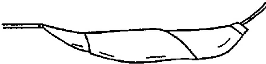
**Fig. 9: Additional Splice Taping**
