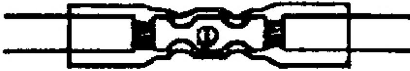
**Fig. 17: Crimped Duraseal Splice Sleeve**
